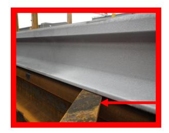
Do not use plain steel bearers when stacking coated rails. Galvanised steel bearers are acceptable if wooden bearers are unavailable
