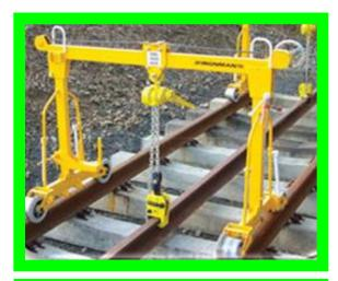
Use tandem lifting hoist system to prevent coating damage during rail movements
