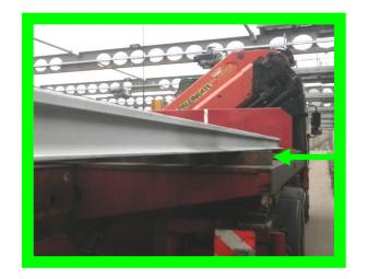
During transportation stack on wooden bearers to prevent impact damage
