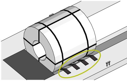
✓ Strips of matting adequately spaced to ensure no contact between the product and the trailer.
