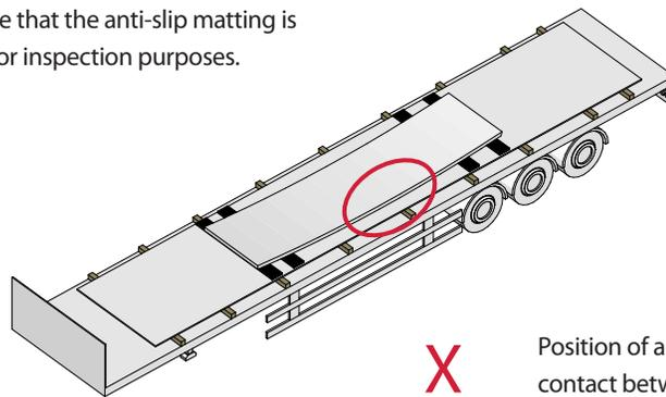
✗ Position of anti-slip matting allows for steel on steel contact between product layers.
