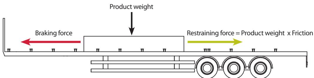
High friction creates more efficient and effective load restraint systems.
