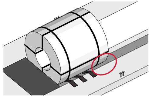
✗ Inadequate and/or poorly positioned anti-slip matting allows product to rest on the trailer bed.
