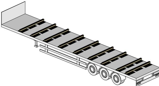
✓ Anti-slip matting must be applied on top and beneath each timber bearer to avoid sliding of the product and timbers across the trailer deck.
