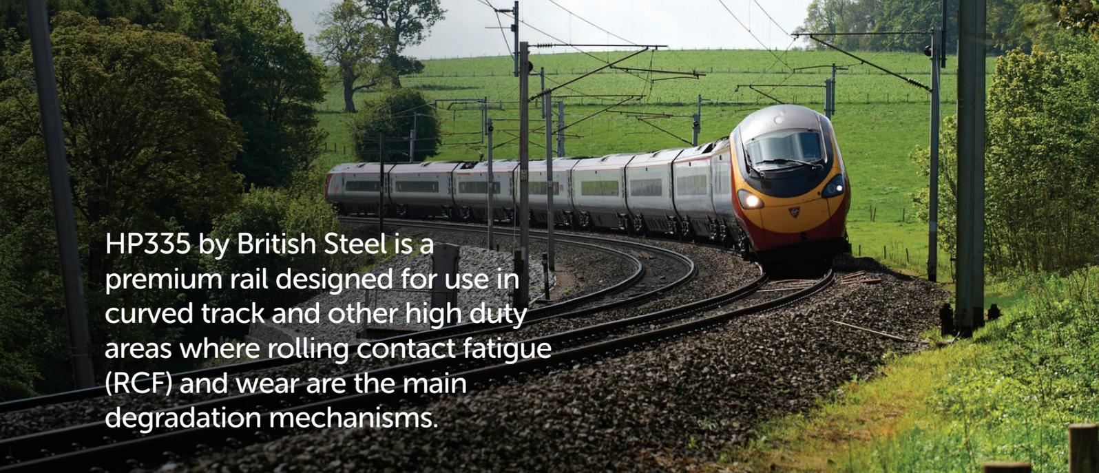
HP335 by British Steel is a premium rail designed for use in curved track and other high duty areas where rolling contact fatigue (RCF) and wear are the main degradation mechanisms.
