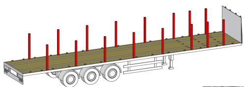
Telescopic stanchions can be used with wide products, thereby providing blocking for sideways restraint.
